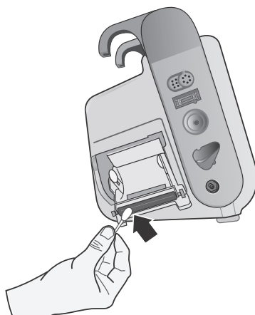
Figure 24-3. Cleaning the Print Head
