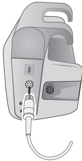
Figure 11-1 Plugging the Transducer into the X Series
