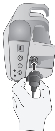
1. Insert MFC into unit.
